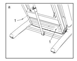
Lower the treadmill (see HOW TO LOWER THE TREADMILL FOR USE on page 27). Remove the four indicated #8 x 3/4" Screws (1), and remove the Motor Hood (75).
